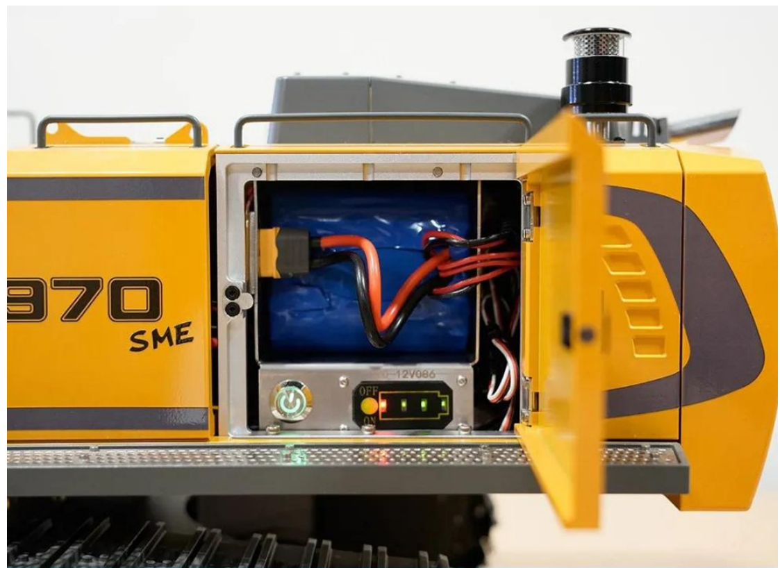
Battery Compartment: Built-in Power Soft Switch And Power Indicator
